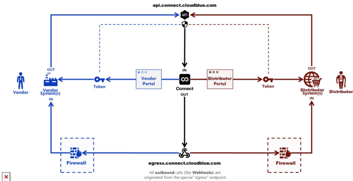
Thus, in case of the firewall configuration being a mandatory requirement for the inbound network connectivity of our partners, you can use that special domain **egress.connect.cloudblue.com** to dynamically retrieve IP address(es) for the inbound firewall rules from **A records** of that domain.
